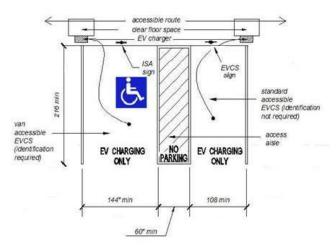
**Floor and ground surfaces** (CBC 11B-812.3): Access aisles shall be at the same level as the vehicle space they serve. Slope not to exceed 1:48.
