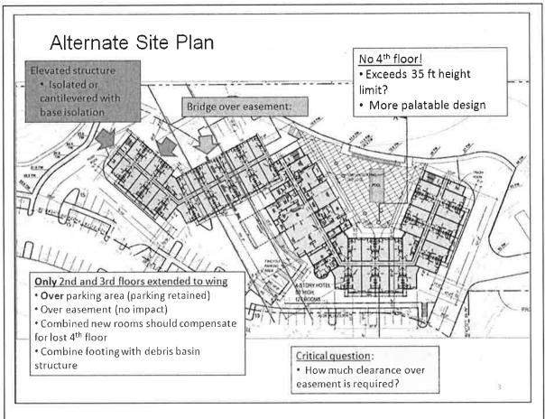
Figure 3. Additional rooms could be added by extending the upper floors of the hotel over the parking lot.
