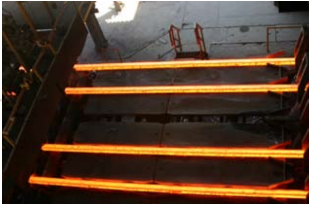
Melted guns being formed into reinforcing bar
