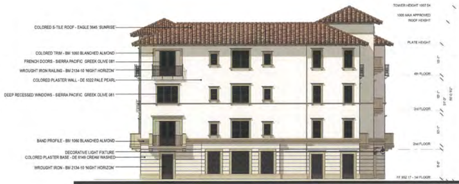
Detail Set 2 LEFT (SOUTH) ELEVATION
