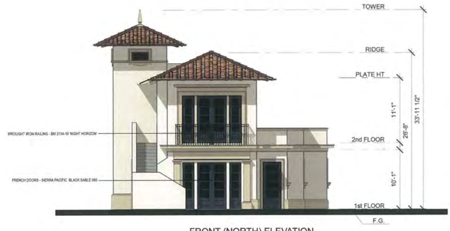
FRONT (NORTH) ELEVATION
