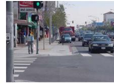
*Mid-block crossing*: A crosswalk designed at a mid-point between intersections. These are usually implemented where there is a long distance between crosswalks on a commercial street.
