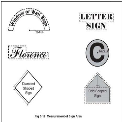
Fig 3-18 Measurement of Sign Area
