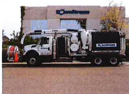
2012 International 7500 - Camel 200 VAC Truck - 10.8 cu.yd unit has 1000 gallon water capacity, 80 GPM @ 2000 PSI water system. This single engine design results in lower sound levels and less fuel consumption* . It allows the vacuum, water and hydraulic pumps to operate efficiently while transmission is In Neutral. Back flushed debris is vacuumed from the manhole/catch basin, water and solids are retained by the collector body, liquid is separated from debris by the ejector plate and removed via the front body drain.
