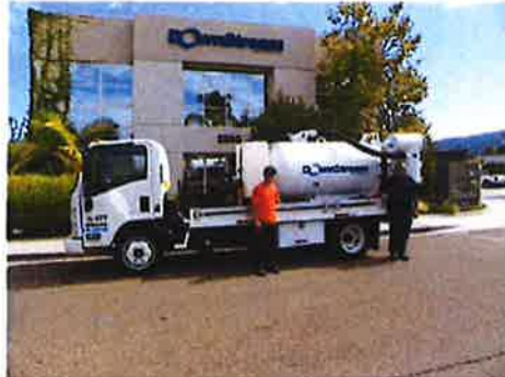
2015 Isuzu Storm Drain VAC Cleaning Truck with Vermeer Vactron Deutz 3 CYL and 500 gallon debris tank with hydraulic lift dump - 1000 cfm vacuum pump capable of 15" of mercury. Hydraulic Components are operating with non-toxic, zinc-free bio degradable hydraulic oil*
