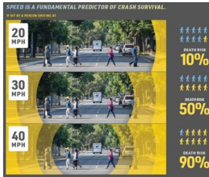
Figure 2.3 Increasing driver vehicle speed reduces vulnerable road user crash survivability and narrows the driver's field of vision.
