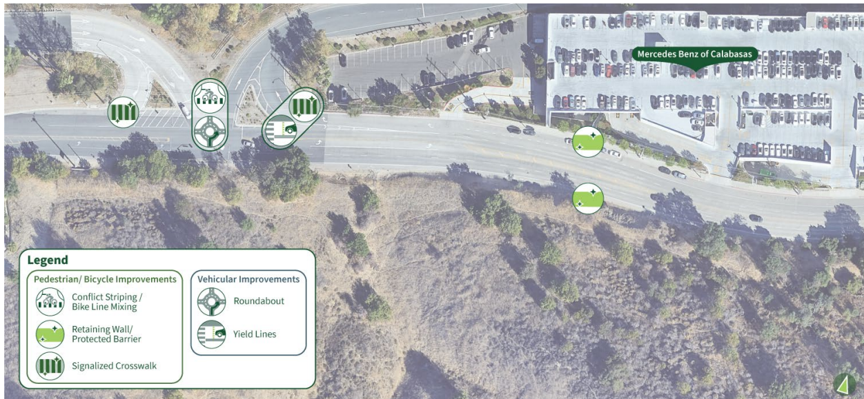
Figure 5.5 Calabasas Road and 101 Freeway Interchange Recommendations Overview
