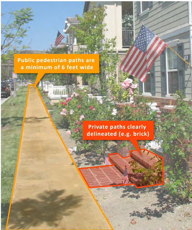
Figure 10: Pedestrian paths on private property are clearly delineated with colored concrete. (Section: 3.1.1.B)
