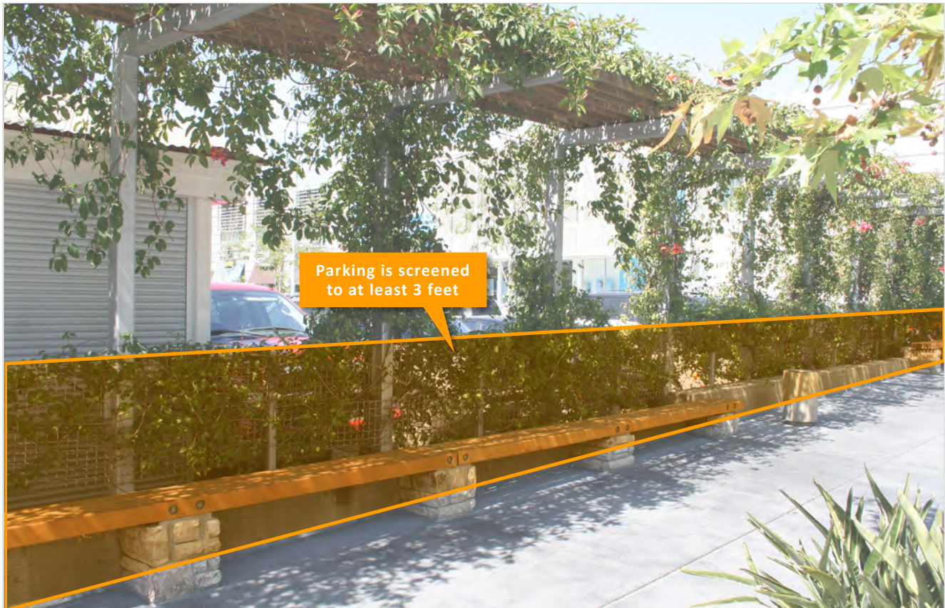
Figure 15: The parking area is screened from view from the adjacent primary street with a three (3)-foot-high landscaped hedge. (Section 3.2.1.C)
