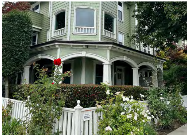
Figure 71: Residential ground floor unit entries shall incorporate at least an additional three-foot landscaped setback or be elevated at least two feet above sidewalk level. (Section 7.5.1.C)
