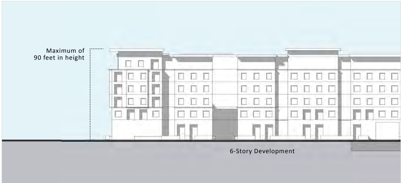
Figure 4: Mid-rise shall mean buildings between four (4) and seven (7) stories but not more than ninety (90) feet in height. (Section 2.2.H.B)
