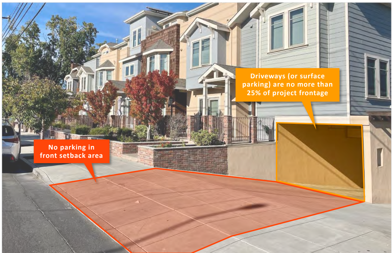
Figure 14: Parking and driveways shall occupy no more than twenty-five (25) percent or sixty (60) feet of the project frontage, whichever is greater. (Section 3.2.1.B)
