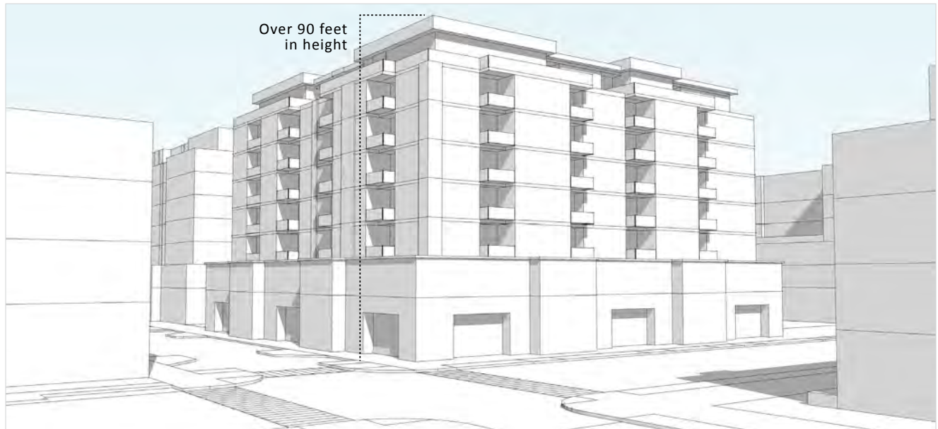
Figure 7: High-rise shall mean buildings eight or more stories or greater than ninety (90) feet in height. (Section 2.2.H.C)
