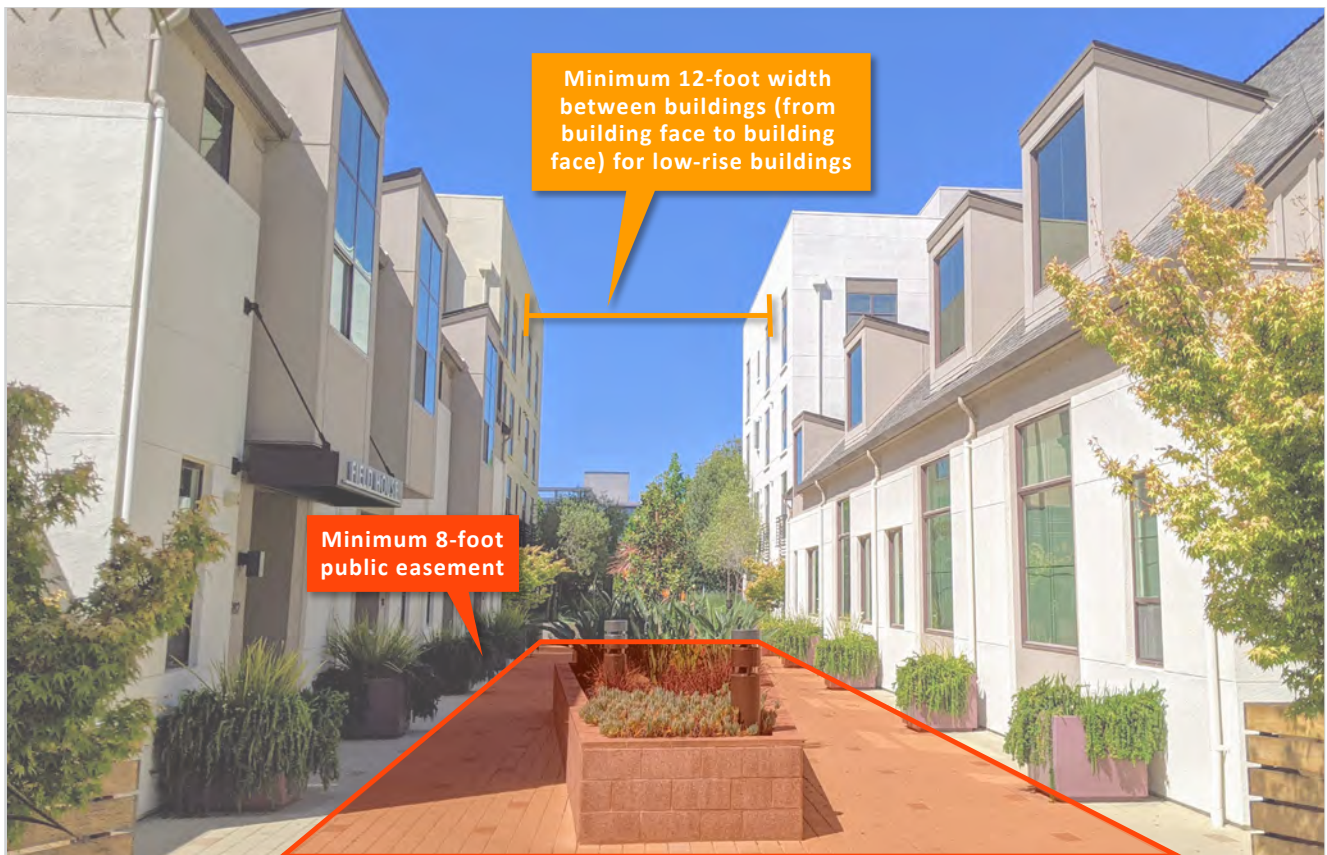
Figure 12: A pedestrian paseo between low-rise buildings has a minimum eight (8)-foot-wide public access easement and a minimum twelve (12)-foot width, as measured from building face to adjacent building face. (Sections 3.1.2.B and 3.1.2.D)
