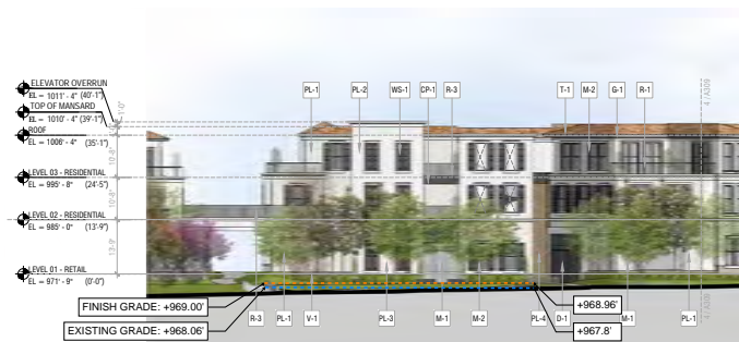
3 Building B-2 North Elevation SCALE: 1/16"=1'-0"
