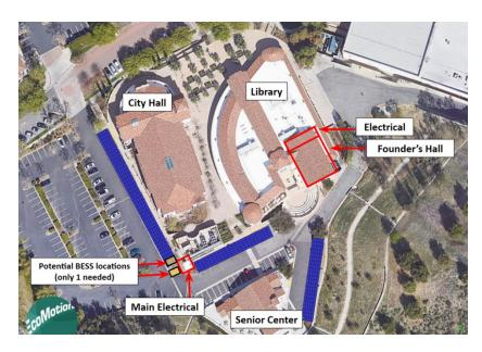
• Option 2 is a 270-kW combination solar carport and rooftop solar array projected to generate approximately 430,000 kWh / year, which accounts for approximately 48% of the campus' annual use of 900,000 kWh.
