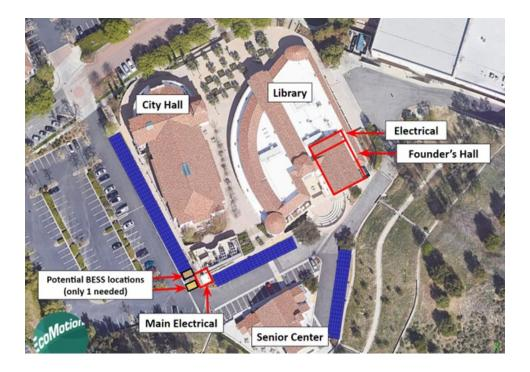
The carports combine to equal approximately 165 kW of PV panels, which is projected to generate 275,000kWh annually. The annual usage of the entire campus is 900,000 kWh, but the annual usage of Founder's Hall is but a fraction of this. The entire campus is on a single meter.
