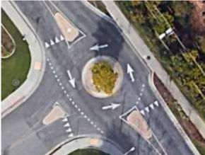
Description: A raised circular island placed in the center of an existing local street intersection, thus creating a roundabout. A roundabout allows for more efficient right-of-way allocation at higher volume intersections and typically found on collector streets in place of a traffic signal Both roundabouts and traffic circles force drivers to meander around the raised island which prevents speeding through the intersection.
