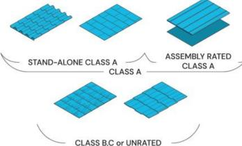
Roof covering fire ratings are Class A, B, C, or unrated; with Class A providing the best performance. Common Class A roof coverings include asphalt fiberglass composition shingles, concrete and flat/barrel-shaped tiles. A roof can achieve a Class A rating on its own (stand-alone Class A) or when combined with other fire-resistant elements (assembly-rated Class A).
