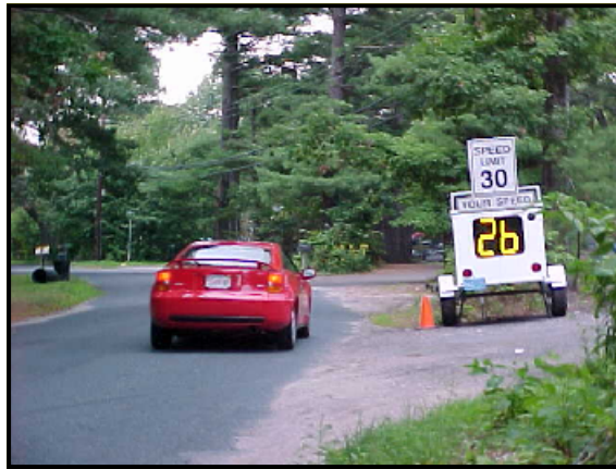
Sample Speed Monitoring Device
