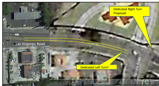
Fig. XVI-1. There may be room enough in the as completed center divider to create a dedicated left turn storage lane.
