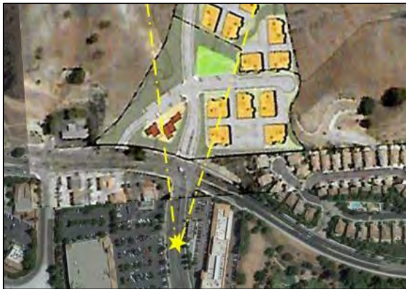
Figure I-3. Locating the rendering point of view by triangulation, using identifiable landmarks for reference. [Credit: New Homes and Google]
