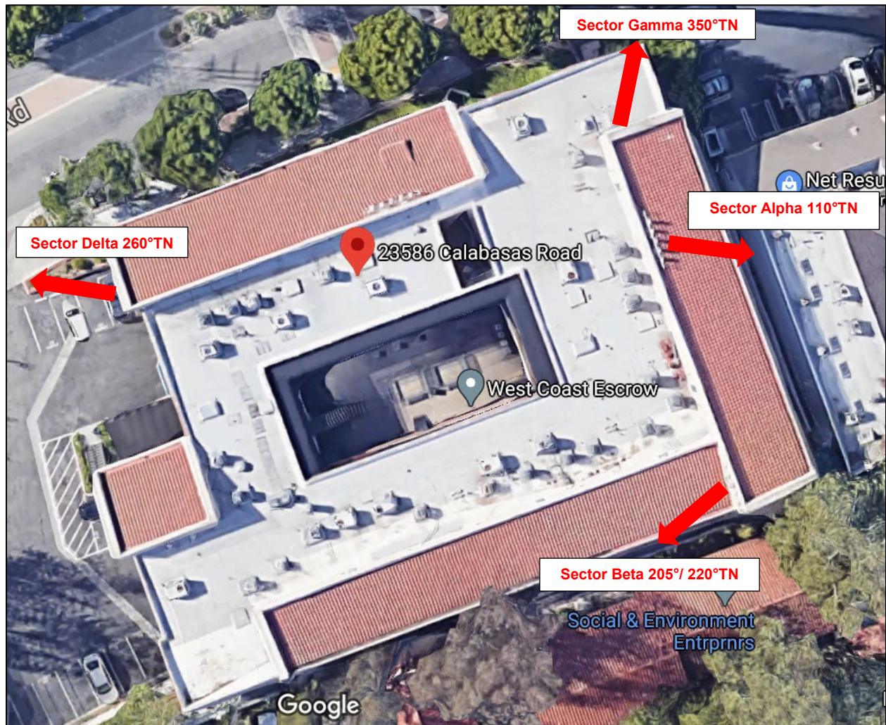
Figure 1: Overview of approximate sector locations for antennas (Source: Google Overview, annotations by Dr. Kramer).
