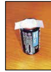
Step 2: Place tape on positive (+) end
